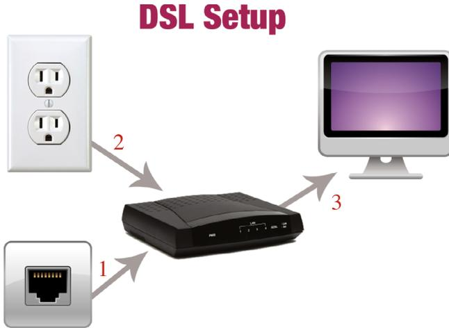
1. Plug one end of the phone cord into the phone jack and the other end into the modem
